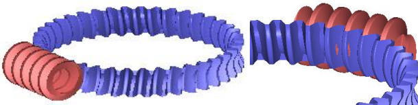
Fig 3.70 [3]Cylindrical worm gear
